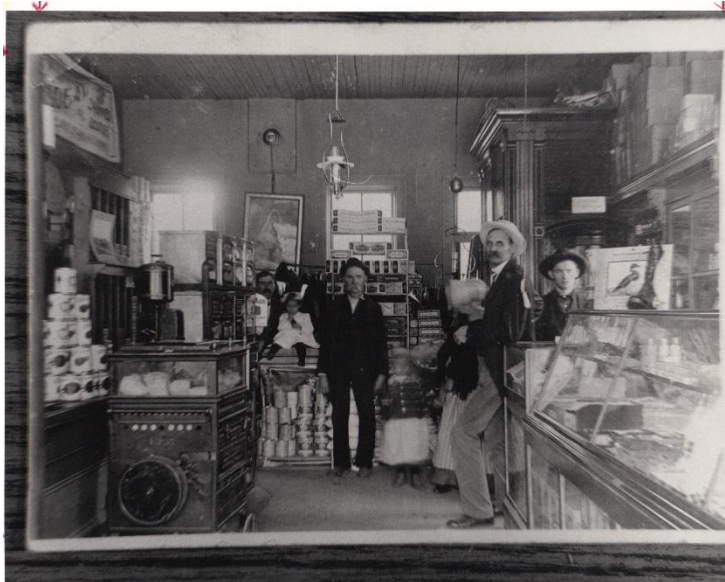
The equipment directly above is a peanut roaster and popcorn machine. The white box above it is a container of "white" gasoline, used to heat the roaster. Do you remember those old fans in stores before air conditioning became the norm?
